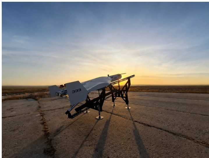
Figure 1. MICH 2000 on a launch rail; image retained from the source report.
