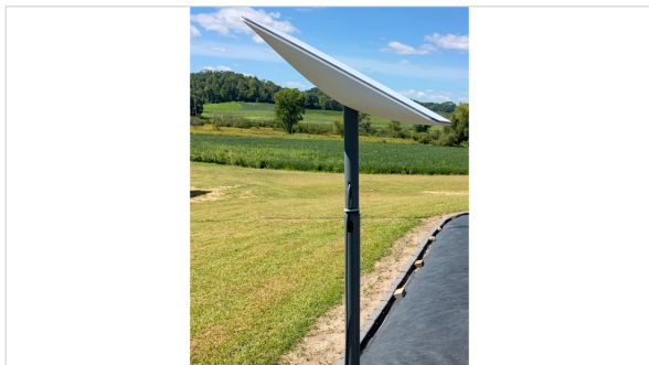
FIG. 7 | Pole-mounted commercial Starlink terminal. Source: Wikideas1 / Wikimedia Commons.
