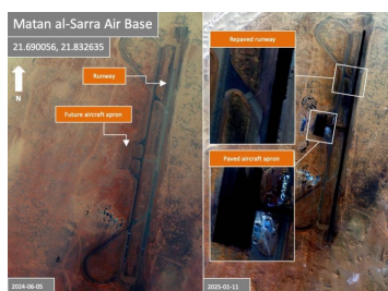
Maaten al-Sarra Air Base: runway repaving and new aircraft apron, 2024-2025. Source: Tearline analytical imagery / commercial satellite imagery
